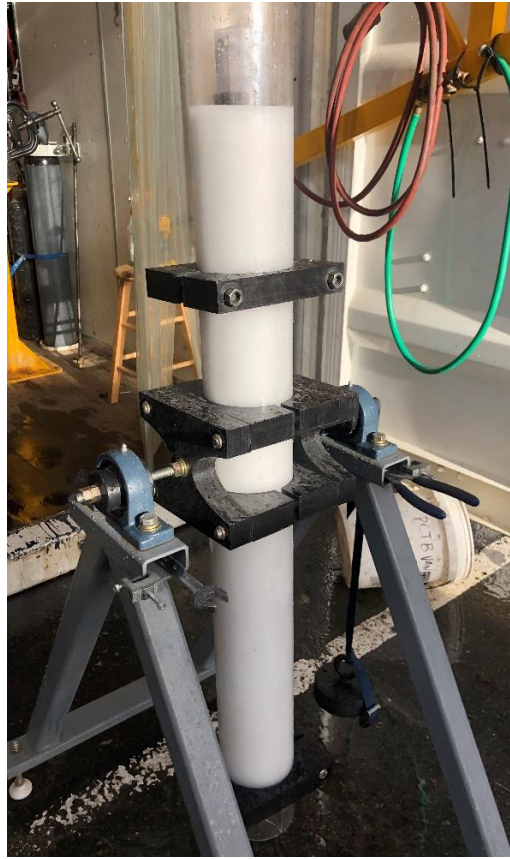
Figure 1. Ball valve assembly in test fixture with Min-U-Sil and water solution
